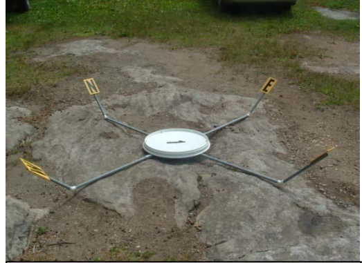
22. Underwater compass targets (shown here on land), placed in various locations in the lake, allow photos taken over time to be compared for milfoil and native spread. A Vermont DEC idea for simplifying plant surveys.
