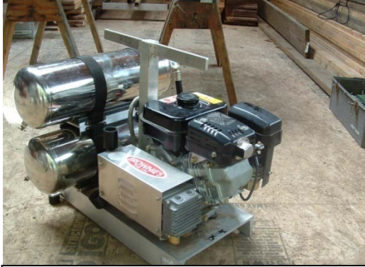
7. The hooka air compressor, expensive, but well worth it. It could safely support 4 divers and operate all day on a tank full of gas.
